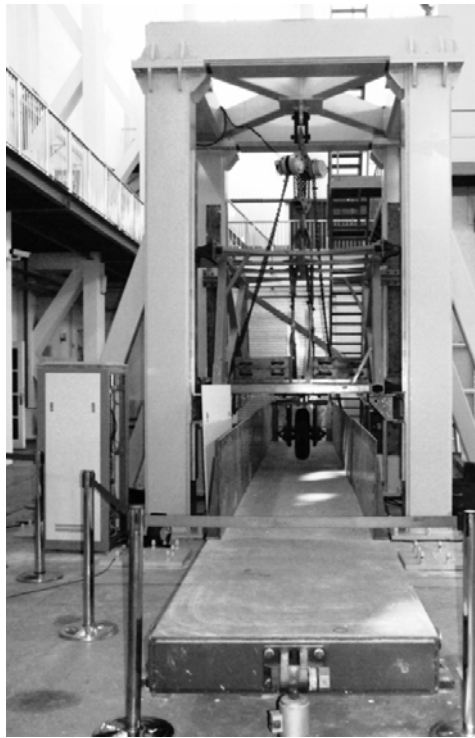
Figure 6. The apparatus for single-wheel load experiment
